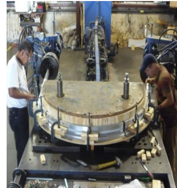
Stretch form press curving a pre-anodized store front shape Capable of up to 200 degrees of arc.
